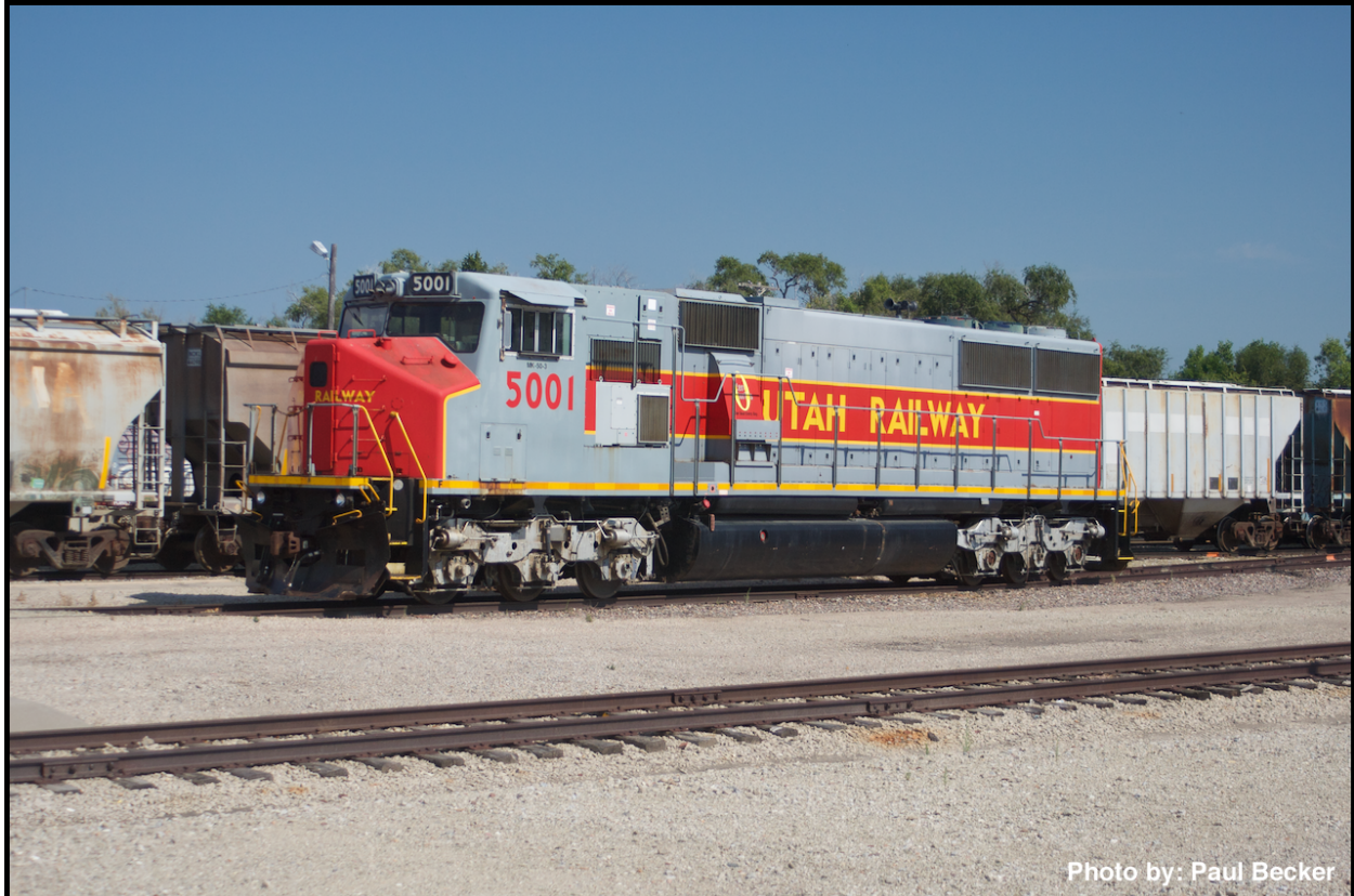
(Utah Railway #5001 MK-50-3 Built 8/94 as SP MK5000C #501. Rebuilt to MK-50-3 July-September 2003 for Utah Railway by MK/Boise Locomotive.) Phillipsburg, KS.
